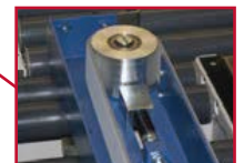
Self-tensioning & tracking side drives simplify belt replacement
